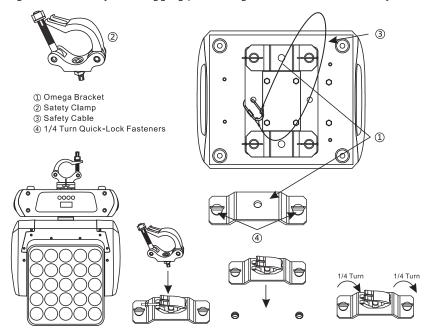
Regardless of the rigging option you choose for your MADPANEL 2510F, always be sure to secure your fixture with a safety cable. The fixture provides a built-in rigging point for a safety cable on the hanging bracket as illustrated above. Be sure to only use the designated rigging point for the safety cable and never secure a safety cable to a carrying handle.
